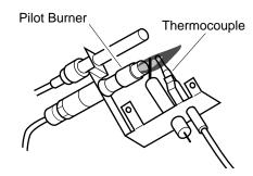
Figure 29 - Correct Pilot Flame Pattern
